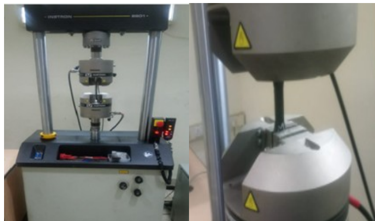
Fig.2. (a) shows the universal testing machine for testing tensile specimens.(b) shows the tensile specimen in the machine
