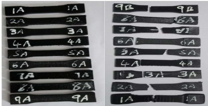
Fig.1. (a) shows the fabricated tensile specimens before a test. (b) Shows the fabricated tensile specimen after the test.
