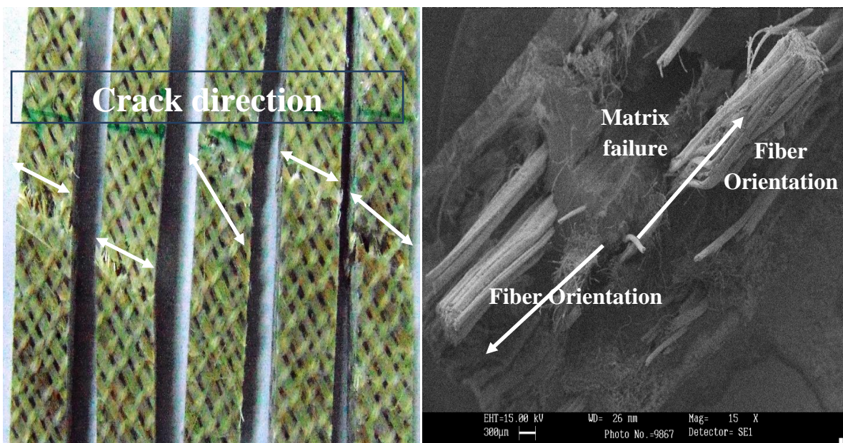
Fig. 9: Fractured specimen and SEM image of surface of inclined cross plied SFRP
